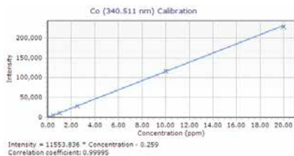
Figure 1. Typical linear calibration curve for Co at the 340.511 nm wavelength
