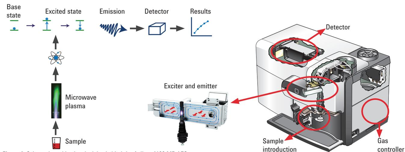
**Figure 1.** Schematic and basic principles behind the Agilent 4100 MP-AES
